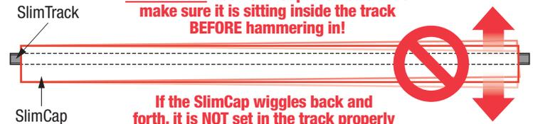
**If the SlimCap wiggles back and forth, it is NOT set in the track properly and will be damaged when hammered in!**
