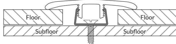
4. Starting at one end, press the molding into the track inching along the length of the molding.
