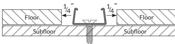
3. Center the track between the flooring leaving a 1/4" spacing between the track and floor planks. Screw track to subfloor (or glue down with construction adhesive).
