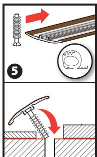
Slide dowels into groove on bottom of the SlimTrim molding and position them according to template. Line up dowels with pre-drilled holes. Adjust dowels as needed.
