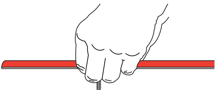
**NOTE:** Do not try to push the entire molding in all at once by just pressing it in from top! This will bend the dowels.
