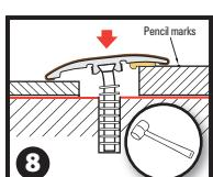
When finished applying adhesive, start again at beginning of molding and push dowels all the way down until molding is secure. Use a rubber mallet to gently tap on top of each dowel until molding sits flush. Use pencil marks as reference.
