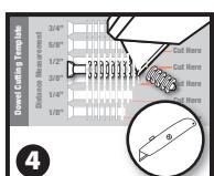
With dowel on template, use a utility knife to cut dowel as indicated on **Dowel Cutting Template**. Repeat with all dowels that are to be used.
