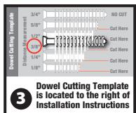
Carefully cut or break dowels from Dowel Tree. Use the **Dowel Cutting Template** to the right to find your measurement on the template and lay your dowel over the number that matches your distance measurement.
