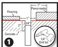
Install flooring planks, leaving 1 inch gap for molding installation. Draw line on flooring for hole placement. Using a 1/4" concrete drill bit pre-drill 2" deep holes using same measurements as dowels. With pencil, mark on floor the location of each dowel. **BE SURE TO VACUUM PRE-DRILLED HOLES.**
