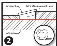
Lay a flat object over flooring and measure from the concrete at the center between the flooring up to the bottom of your object. This will give you the distance to use on the **Dowel Cutting Template** below.
