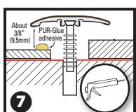
When molding is a finger's width from the floor, insert tip of glue gun under one edge of molding and apply a polyurethane construction adhesive along one side of the flooring. **MAKE SURE YOU APPLY ADHESIVE TO ONLY ONE SIDE OF THE MOLDING AND THAT ALL SURFACES THAT THE ADHESIVE TOUCHES IS DUST AND DEBRIS FREE.**
