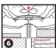
Using both hands, start at one end and gently push molding 1/4" down at a time. It should take several passes to push molding all the way down. Best hand position is holding dowel between pointer fingers and pushing down with thumbs directly over dowel. **DO NOT TRY TO PUSH ENTIRE MOLDING IN ALL AT ONCE.**
